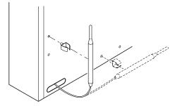
Figure 5 - Moving Thermostat Sensing Bulb
